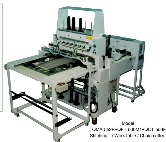
This machine is a compact multiple needle quilting machine developed to serve for the labor saving and possibility of operation without skill as well as sophistication of the stitching department of extra heavy material (Automotive upholstery, furniture, etc.)
