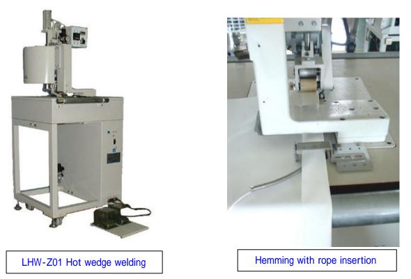
LHW-Z1 has unique designed originally by Queen Light 'Z' shape arm, this 'Z' shape unique arm presents the customers who want to join or hemming wide width sheets easy and efficient work. Both right and left side materials can join with no width limitation, any width material can put through in this
