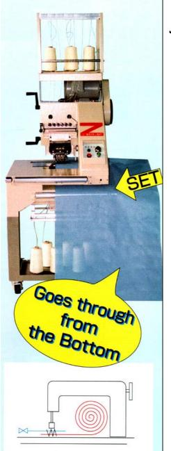
As shown above and left, working on the QMZ machine, right material goes through lower slit of the machine head and left material goes through on the flat bed, therefore any width material can be joined with the machine.
