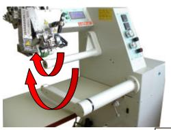
The arm can be interchanged with one lever operation
